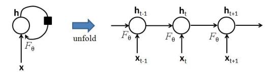
**Left:** Implementation of RNN, viewed as a circuit. The black square indicates a delay of 1 time step. **Right:** the same RNN viewed as an unfolded flow graph, where each node is now associated with one particular time step.
